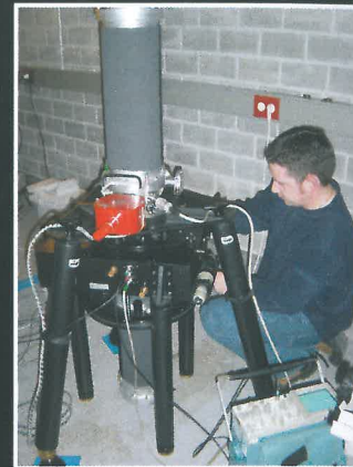
An absolute gravity meter
